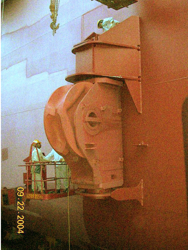
Turndown Sheave and Dual Pawl Chain Stopper for 5" Studless Chain
