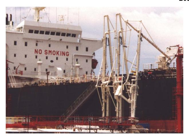
The B0030 Marine Loading Arm is preferred when loading/unloading sea-going tankers and its capability has been proven within many years of trouble free operation world-wide.
