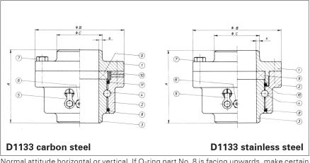
Normal attitude horizontal or vertical. If O-ring part No. 8 is facing upwards, make certain that water cannot enter into O-ring groove (protective cover)
