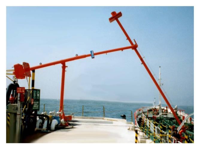
The B0028 Marine Loading Arm is designed especially to meet the needs of barge transfer and coastal tanker installations with minimal tidal variation.
