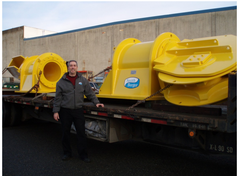
Model 5C-652 Fairlead for Ø3” Chain
