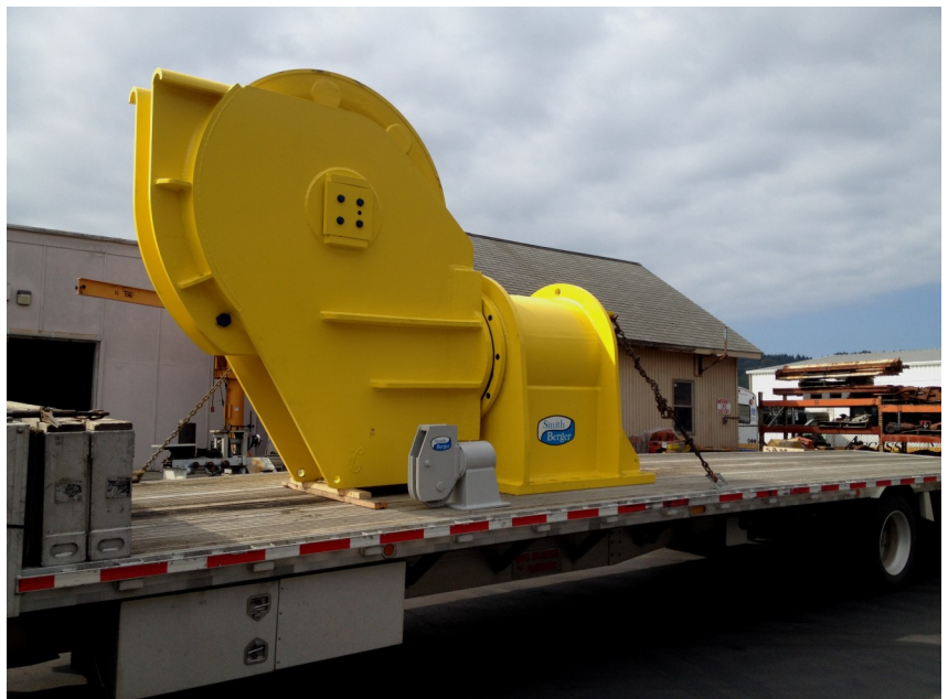
Model MF-874 Fairlead Ø4” Wire Rope SWL 300 Tons
