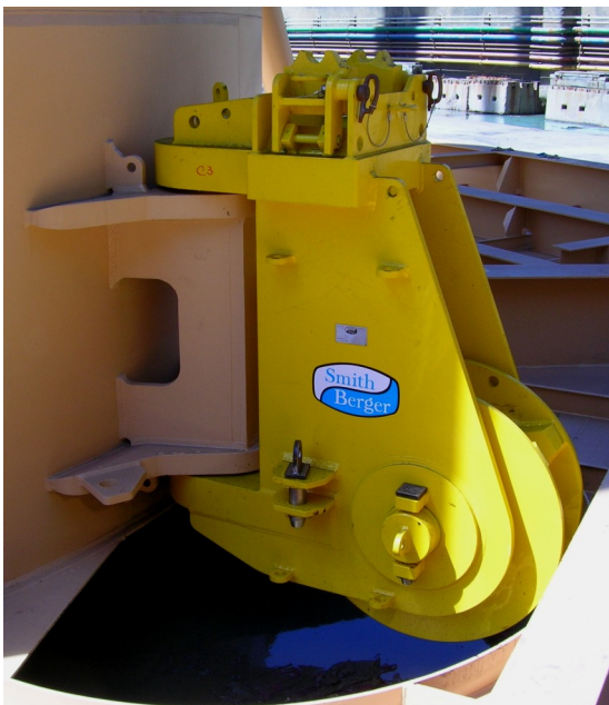
Model 5C-552-CS Underwater Fairlead / Chain Stopper for Ø3” Chain
